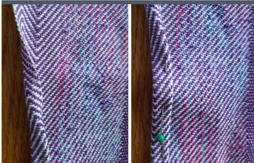
Use Tom's method of treadling a twill hem, and you end up with a hem that perfectly lines up with the rest of the cloth.
