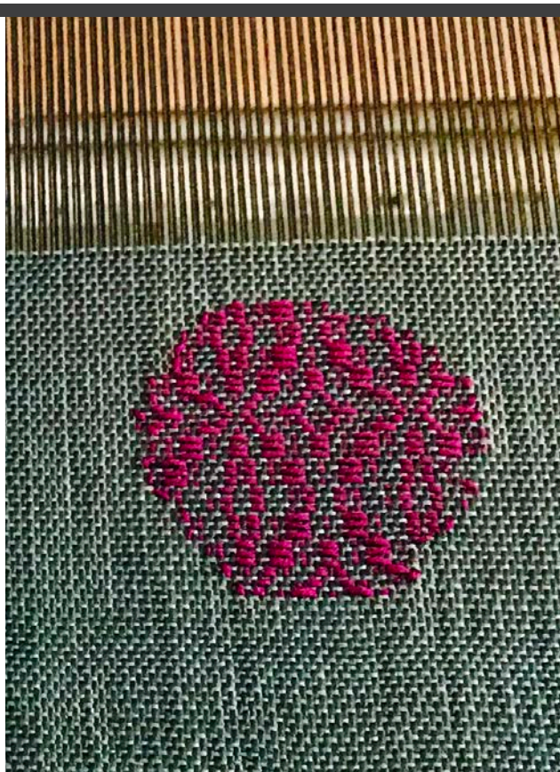
Photo 3. Shapes such as circles can be difficult to weave. They should be elongated on the loom to allow for take-up and shrinkage off the loom.
