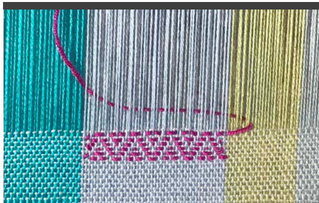
Photo 1. Increasing the width of an inlay area when the shuttle is entering the shed results in a loop.
